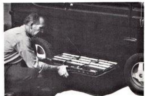
Battery tray slides out for convenient servicing or quick exchange of batteries.
